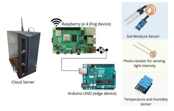
Fig. 3 Soil moisture, temperature, humidity, and light intensity sensors
